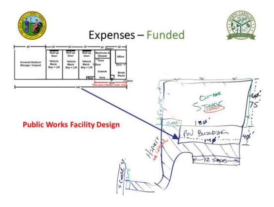
Cordeiro explained the concept. The building structure would be premanufactured 40' x 140'. The left side would include storage where we can park some equipment. There will be three maintenance bays, that will not be airconditioned. The maintenance bays will have lifts in them. The right side of the facility will be airconditioned with cubicle areas, a restroom with shower, an office for the supervisor, and a breakroom / meeting space.
