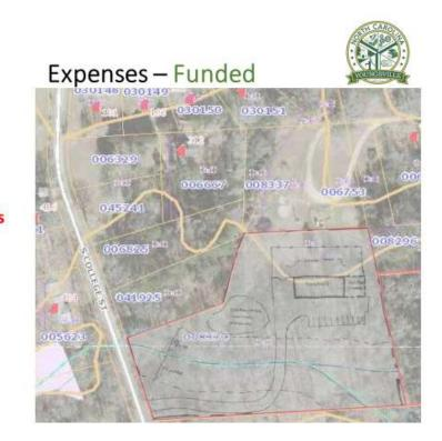
Public Works Facility Site Plan Cordeiro explained the blue line was a stream that had a buffer requirement and there would also be a storm water control pond. He explained the drawing was to scale. When asked, Cordeiro showed the location of the current pump station. Cordeiro explained there would be access and noted we may have to improve the surface, which should not be that expensive.
